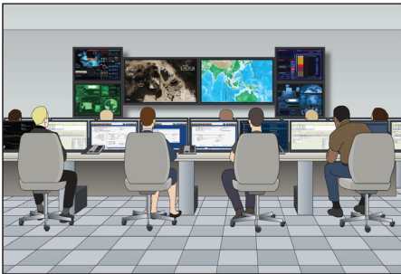
Functioning command center, with a new conductive floor that does not prevent static generation.
