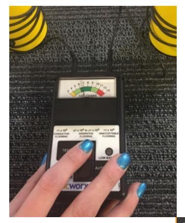
charge to ground. Ground points can be an AC electrical outlet box, an I beam in the building infrastructure or a dedicated rod driven into the earth. **Grounding** a floor (also called *earthing*) requires connecting the antistatic floor to a point in an electrical circuit or building infrastructure that has zero electrical potential. An ESD Ground provides a path for the dissipation of unwanted static electricity charges.
