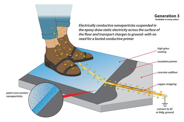
Nano technologies produce fully conductive colorized topcoats (colored and clear). This translates into a floor that requires a standard concrete primer and conductive topcoat.
