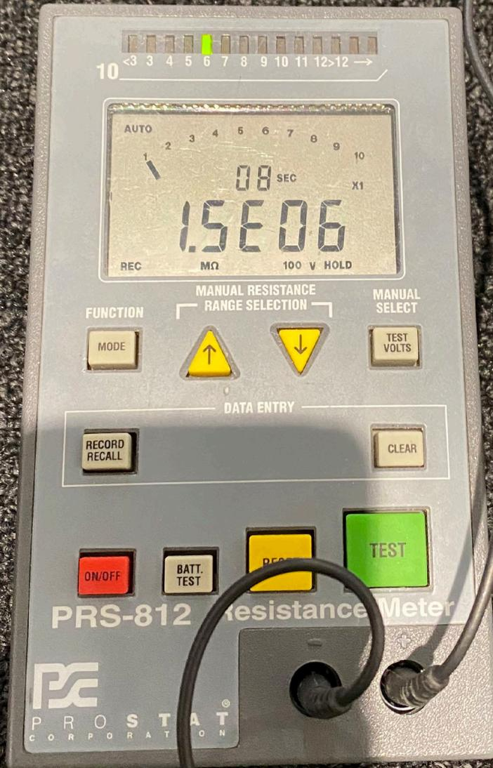
Resistance test measurement, Fields and Stone ESD carpet over raised access floor. Reading:  $1.5 \times 10^6$
