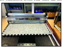
GroundLock tiles can be installed by customers themselves with a bullet cutter, chalk line and dead-blow hammer.
