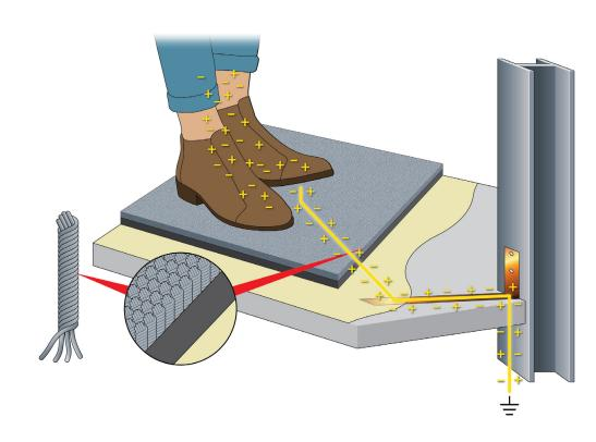
Due to electrical safety risks and compliance with industry-specific grounding standards, conductive flooring is never recommended for schools, networked offices, E-9-1-1 call centers, flight towers or public-access environments. Conductive flooring is usually described as having an electrical resistance between 25,000 ohms and one million ohms. This is sometimes expressed in scientific notation as:  $2.5 \times 10 \text{ E4} - 1.0 \times 10 \text{ E6}$
