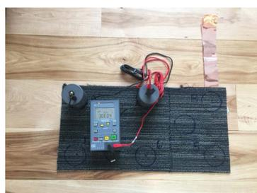
Staticworx™ ESD Carpet has been designed to provide an efficient conductive path-to-ground for static electricity occurring on the surface of the floor (figure E). The electrical resistance range should be 1.0 x 10 E6 - 1.0 x 10 E9 Ohms based on ESD/STM 7.1
