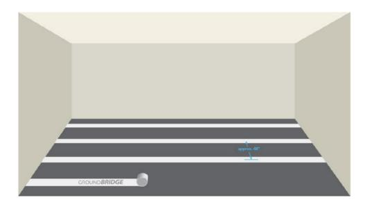
b. Finish installing the GroundBridge underlayment by positioning one strip of GroundBridge along one edge of the room that runs perpendicular to the previously installed strips. This strip will connect all of the ends of the strips, creating a unified ground plane above the subfloor.
