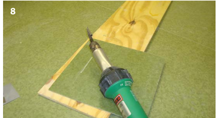
Beginners may find it easier to work with a lower heat. However, with experience, welding will be faster with a higher heat. A lower heat is recommended for correcting mistakes or welding in awkward places. A good weld is achieved when a small amount of melted bead overflows along the edges of the groove.
