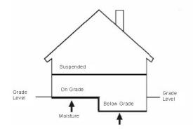
Below Grade – An acceptable below grade floor is a concrete substrate in direct contact with the ground. Properly constructed, the concrete slab will be suitably protected from moisture penetration by planned water drainage and incorporated an effective moisture vapor retarder.
